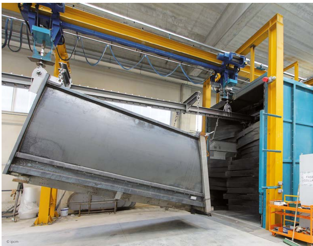
A component entering the shot blasting tunnel and a side view of the shot blasting plant, with 4 of the 16 single-disc turbines.
