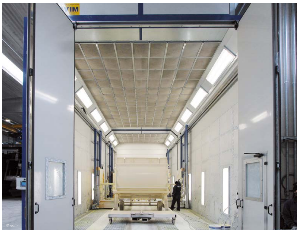
The inside of the manual blasting chamber (above photo) and the inside of the manual coating booth.
