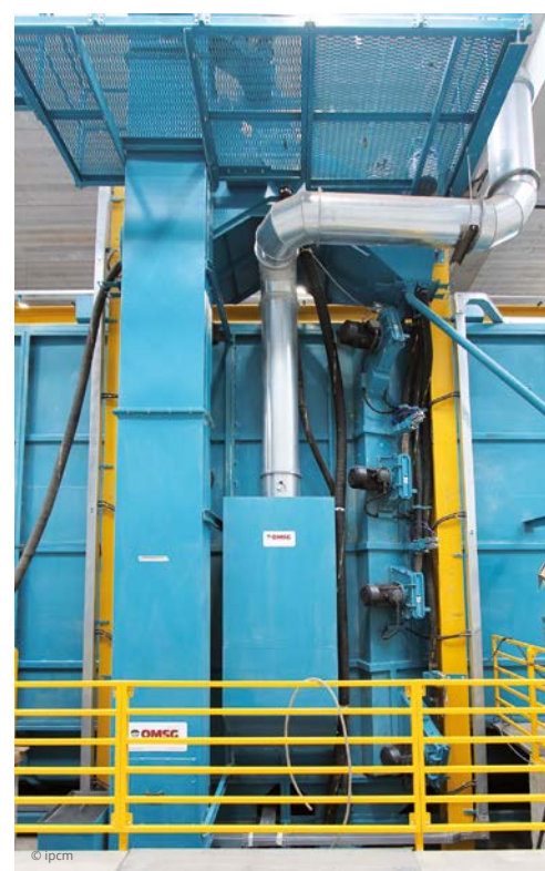
A component entering the shot blasting tunnel and a side view of the shot blasting plant, with 4 of the 16 single-disc turbines.
