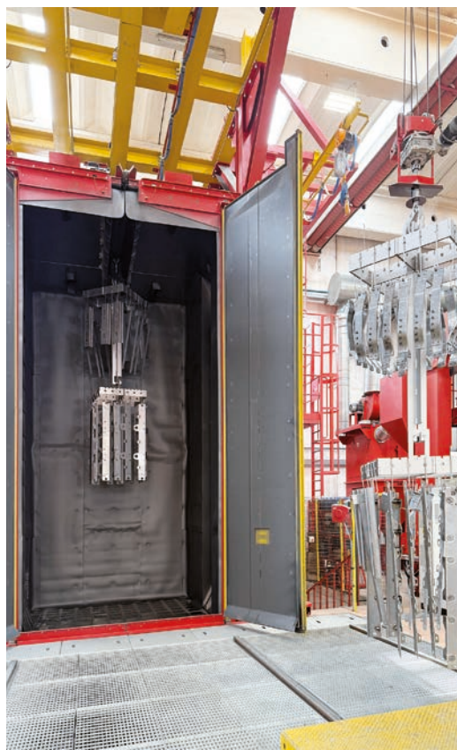
This shot blasting machine is used for medium-sized parts and is equipped with two hoists lifting parts up to 5,000 kg.
