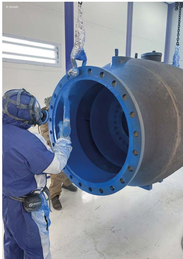
FBE powder coatings call for higher thicknesses than conventional powders.
