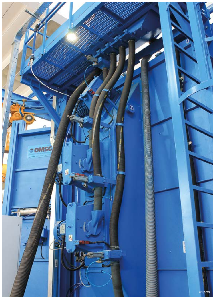
The turbines of the shot blasting machine.
