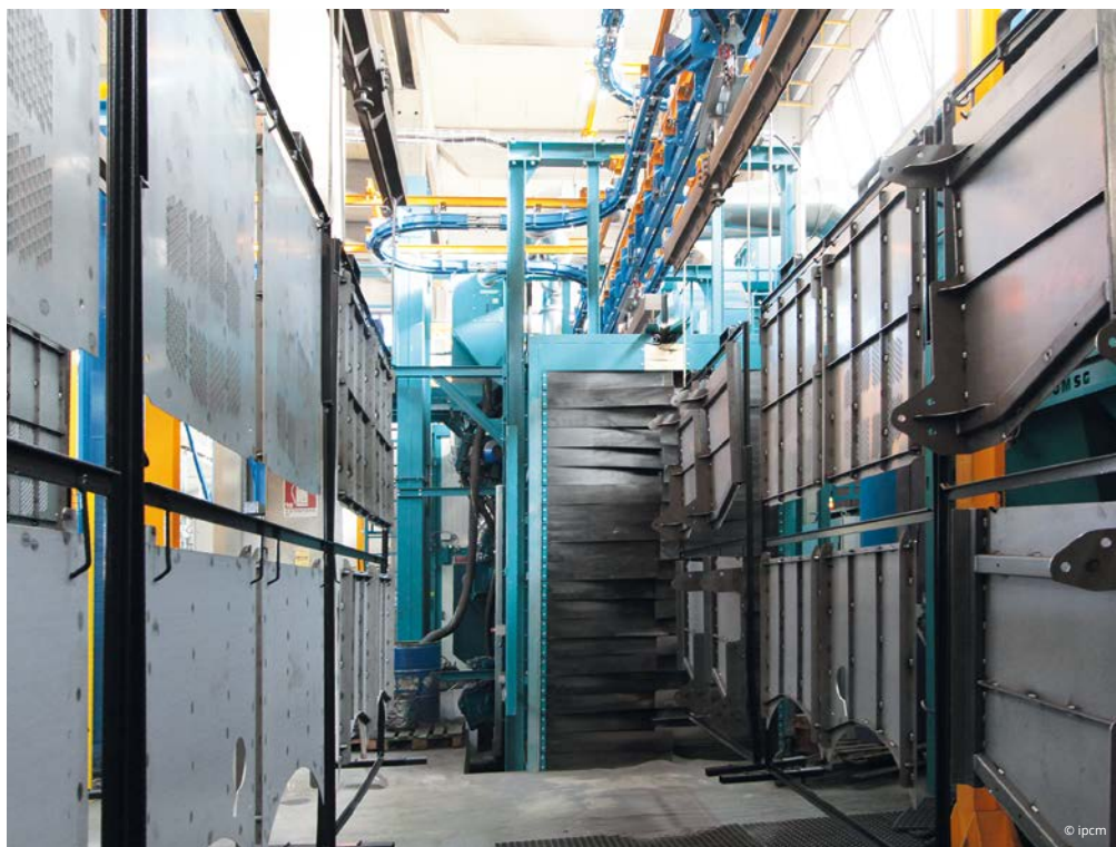
Hung workpieces entering the OMSG automatic tunnel shot blasting machine type TUNNELBLAST 1525/12 SP. OMSG's 12-turbine machine is combined with a 20,000 m³/h self-cleaning filter and it has wear-resistant rubber slats at both the inlet and outlet to prevent metal abrasive from escaping.
