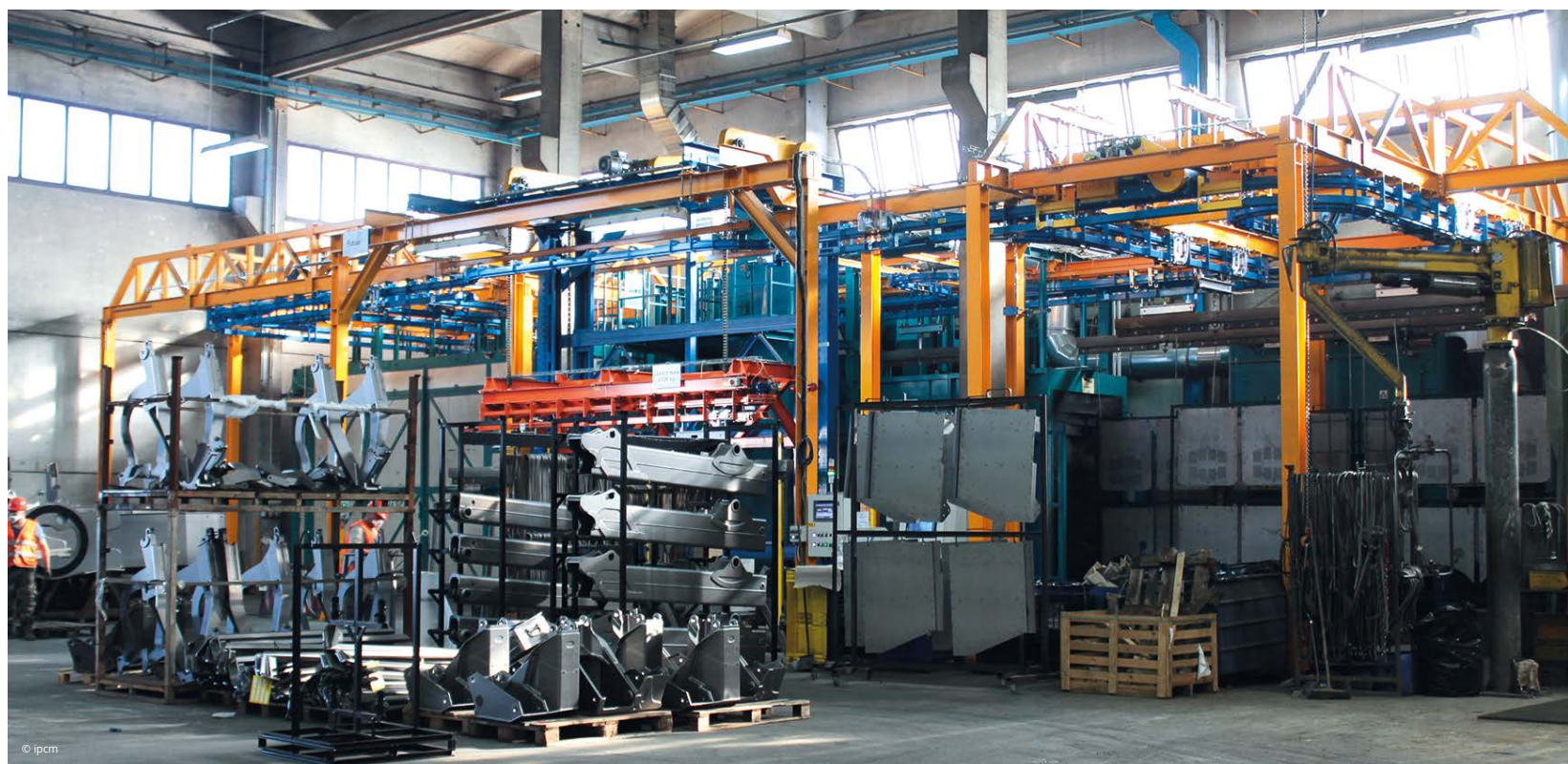
A general view of the new automatic mechanical surface preparation line.
