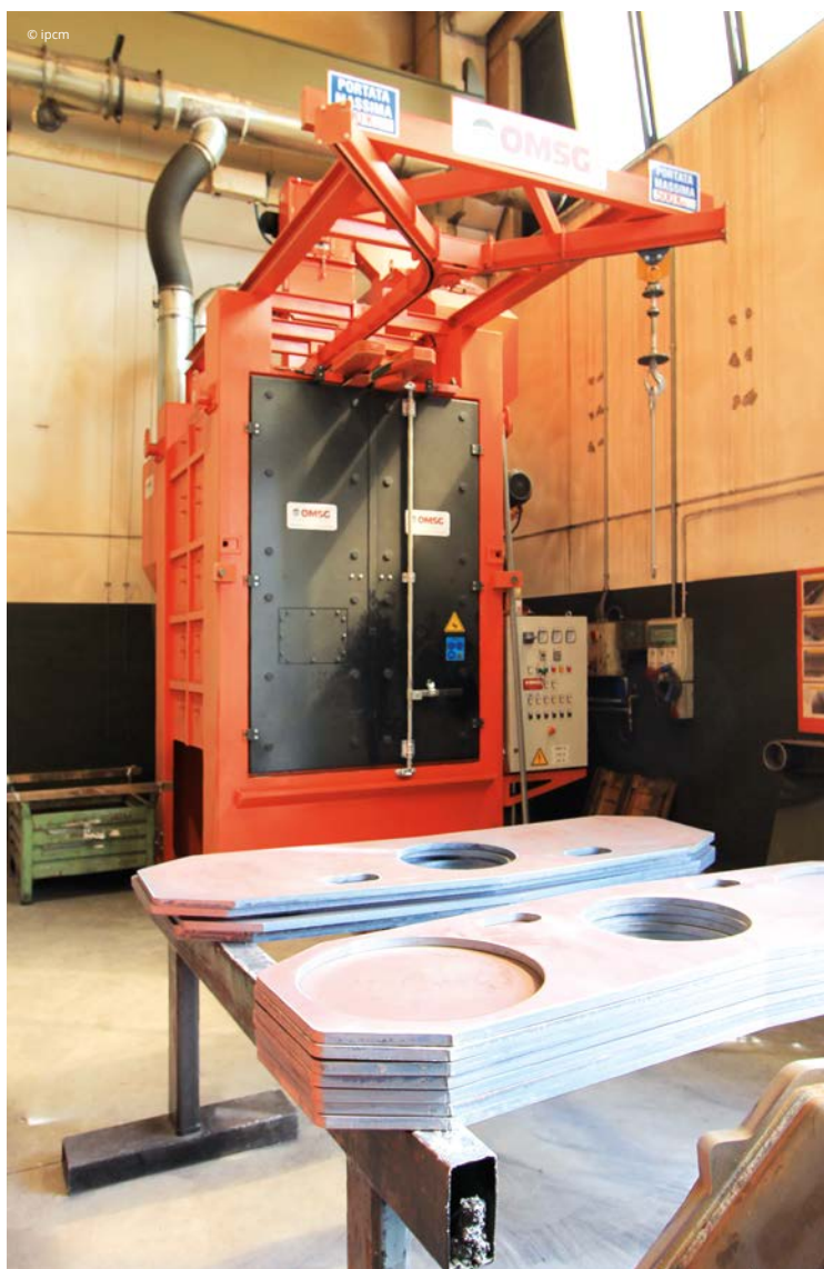
MSG's Dinamo 1216 shot blasting plant.
