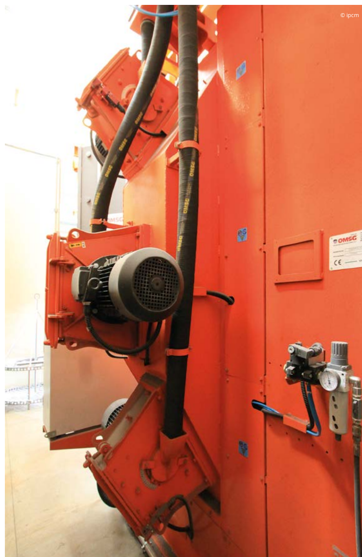
One of the shot blasting machine's turbines.
