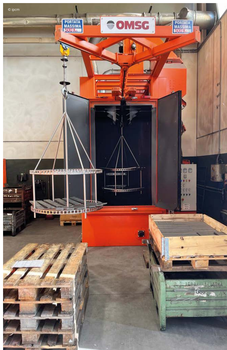
The shot blasting machine with its two hooks for load bar handling.
